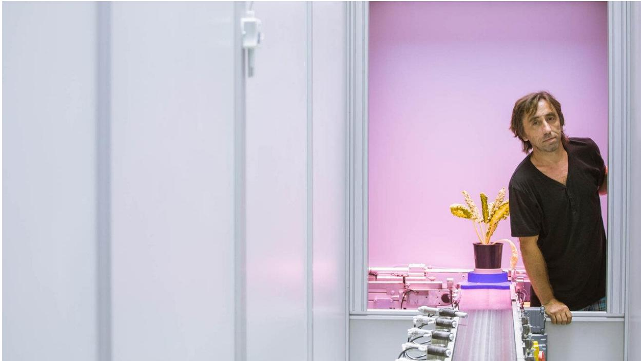
Martin Trtílek with a machine that uses light emitted from plants to determine whether they are stressed, how they are using water and whether they are dying.
